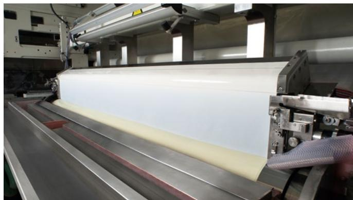
A detailed view on the curtain coating process
