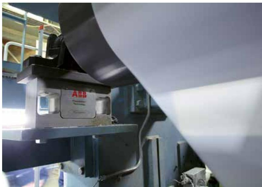
**Web Tension Systems.** A tense situation under full control. Measurement made easy.
